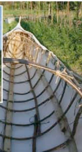
willow & canvas raft designed by Si Holman built by Si & Mac August 2009
